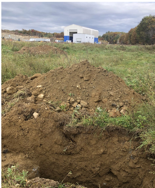
Photo 1 showing sandy/cobbly materials from a test pit. Groundwater is visible in the base of the test pit
