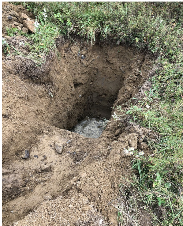
Photo 1 showing sandy/cobbly materials from a test pit. Groundwater is visible in the base of the test pit
